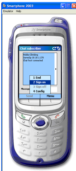
Figure 5. The Smartphone Emulator: The emulator is not the tool of choice to test a distributed application because it does not support callbacks.
